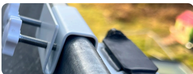
Clamp bracket with two thumbscrews on the front edge of the gutter
